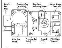
Figure 2 - Dexen Electronic Gas Valve
